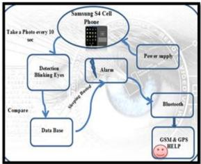
Fig.4 The block diagram for the system
